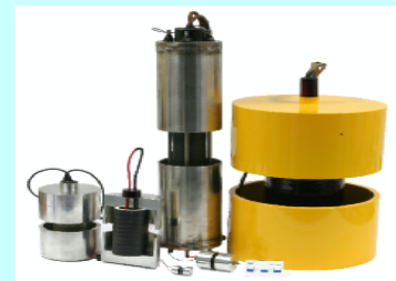
L-R mid-frequency cut-away, extreme high frequency, high frequency & low frequency MMPP's
